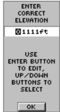
The 'ENTER CORRECT ELEVATION' Page allows you to change the elevation for the waypoint.
