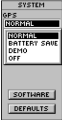
Turn the GPS receiver off to conserve power when using as a compass or developing a pressure trend.
