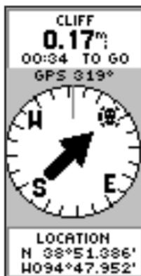
The pointer tells you what direction you should move. When the pointer is pointing right as shown here, just move right until the pointer is pointing straight up and points to the moving direction line (see picture below).
