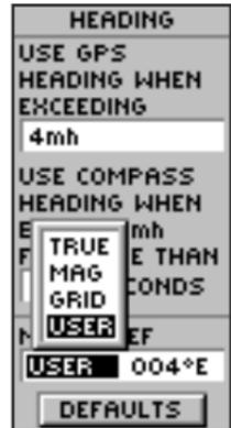
The eTrex Summit automatically adjusts the declination. While it should rarely be needed the user can manually adjust the declination.
