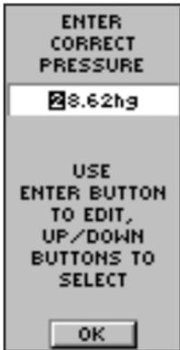
*The eTrex Summit can try to automatically calibrate the altimeter using GPS altitude readings. For optimum performance of the Altimeter you should perform the calibration procedure entering either the correct elevation or barometric pressure.*
