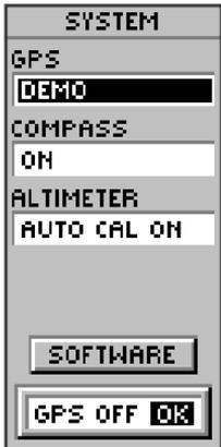
When the unit is in 'DEMO' mode, a warning will appear indicating that the GPS receiver is turned off.
