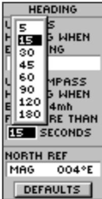
Set a time delay before switching to the electronic compass when moving at a speed slower than the user-selectable speed.
