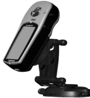
*While mounted in a car or on a bicycle the eTrex Summit will be tilted enough for the Electronic Compass to become inaccurate. The eTrex Summit will automatically switch to a GPS heading when you exceed 10 mph. To switch back to the compass press and hold the **PAGE** key or wait 90 seconds after slowing below 10 mph.*
