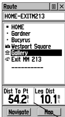
Distance to Point vs Leg Distance. To view Leg information, highlight the end waypoint on a leg.
