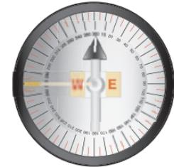
The Geko 201 is not a true magnetic compass! You must be moving in order for it to track your movement.
