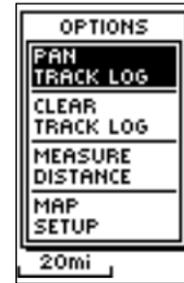
Selecting 'PAN TRACK LOG' from the Map Page options allows you to move the pointer to any point on the track log and then create a Waypoint or navigate to it.
