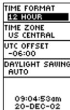
The Setup Page allows you to customize the Geko 201. On the Setup Page you can change coordinate systems, map datums, and distance units. You can also change the time format, north reference, operating mode, display contrast, and back light timeout setting.
