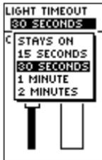
The Light Timeout options allow you to set the backlight to stay on all the time, but watch the battery power!
