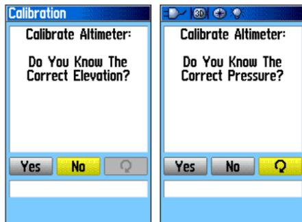
4. Use the **ROCKER** to enter the new elevation or pressure, then highlight **OK** and press **ENTER** to return to the Altimeter Page.
