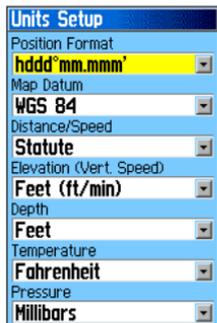
**Position Format**—the coordinates for the system in which a particular location is shown. The default format is latitude and longitude in degrees, minutes, and thousandths of a minute (hddd°mm.mmm).
