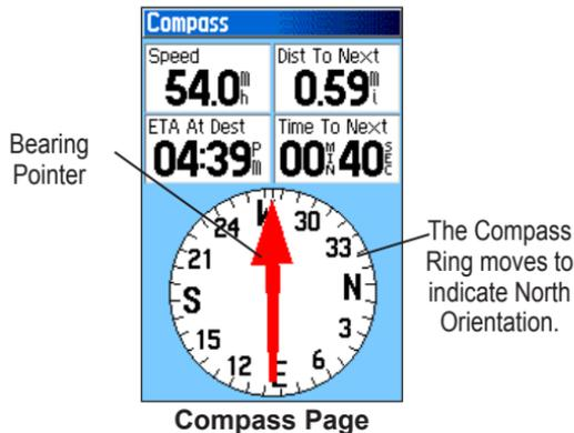
When navigating, the Compass Page provides navigation data and directions. It uses a graphic compass ring, a bearing/course pointer and digital data fields to show information such as current speed, distance to the next point on the route, estimated arrival time.
