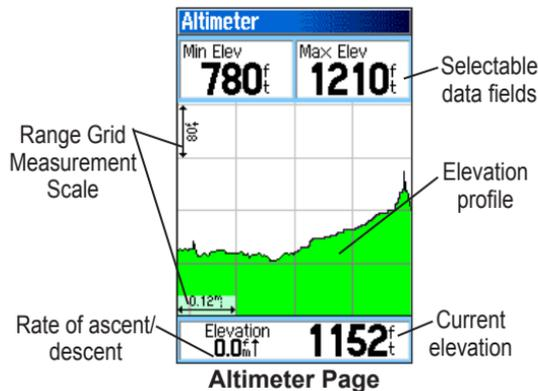
The Status field at the bottom of the page shows the current elevation and your current rate of ascent or descent when moving. It can also show the ambient pressure and time of measurement.
