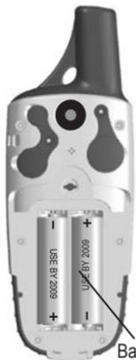
1. Remove the battery cover by turning the D-Ring 1/4 turn counter-clockwise and pulling the cover loose.
