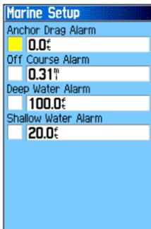
**Anchor Drag Alarm**—sets an alarm to sound when you exceed a specified drift distance.
