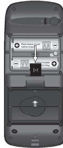
The GPSMAP 76Cx requires two AA batteries (not included), which are located in the back of the unit under the D-Ring. Alkaline or NiMH batteries can be used (see the *Owner's Manual* for setting the battery type). Stored data is not lost when batteries are removed.
